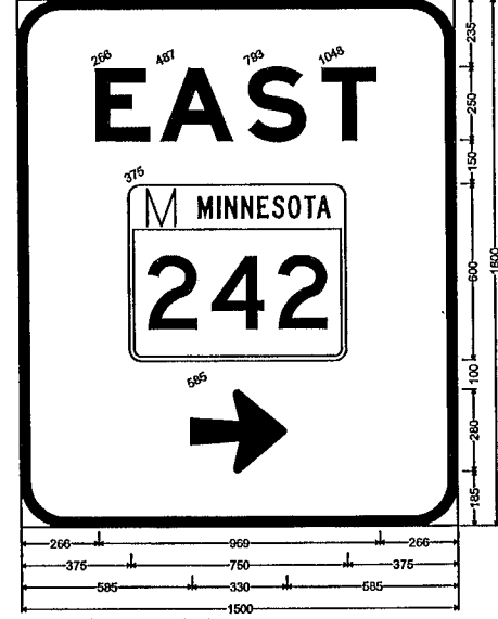
152mm Radius, 32mm Border, White on Green; [EAST] E Mod; Arrow 5 - 330mm 0°;
