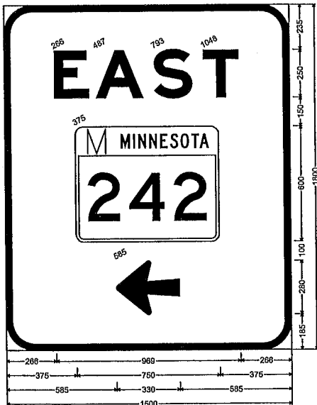
152mm Radius, 32mm Border, White on Green; [EAST] E Mod; Arrow 5 - 330mm 180°;
