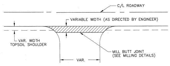
NOTE: KICKOUT PAID FOR AS ITEM NO. 2350.609 (TYPE MV 4 WEARING COURSE MIXTURE)/ OR KICKOUT PAID FOR AS ITEM NO. 2350.604 (TYPE MV 4 WEAR COURSE 1 1/2" THICK)
