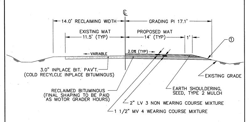
1) STRIPPING OF INPLACE TOPSOIL PRIOR TO WIDENING IF REQUIRED AND AS DIRECTED BY THE ENGINEER, TO BE PAID AS MOTOR GRADER HOURS.
