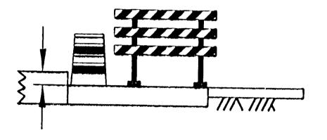
LANE SHALL BE CLOSED WITH APPROPRIATE LANE CLOSURE FROM APPENDIX B. CHANNELIZING DEVICES AT A MAXIMUM OF 100 FT. SPACING AND A TYPE III BARRICADE EVERY 1000 FT.
