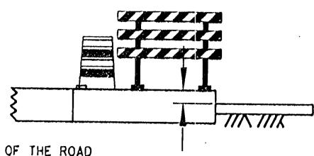
NOTE: SIGNS ARE REQUIRED ONLY ON THE SIDE OF THE ROAD THAT IS AFFECTED BY CONSTRUCTION (EXCEPT SIGNS THAT ARE FOR A LANE CLOSURE ON DIVIDED HIGHWAYS).
