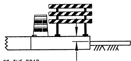
NOTE: SIGNS ARE REQUIRED ONLY ON THE SIDE OF THE ROAD THAT IS AFFECTED BY CONSTRUCTION (EXCEPT SIGNS THAT ARE FOR A LANE CLOSURE ON DIVIDED HIGHWAYS).
