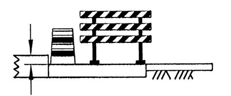
LANE SHALL BE CLOSED WITH APPROPRIATE LANE CLOSURE FROM APPENDIX B. CHANNELIZING DEVICES AT A MAXIMUM OF 100 FT. SPACING AND A TYPE III BARRICADE EVERY 1000 FT.
