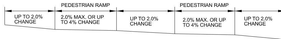
FLOW LINE PROFILE "TABLE" - TWIN PERPENDICULARS
