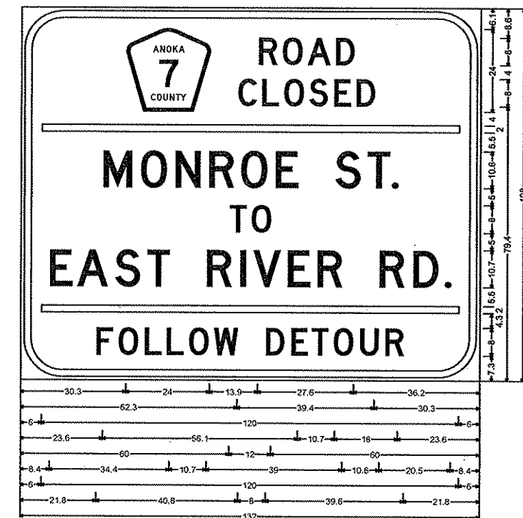
G20-X2_132x108; 12.0" Radius, 2.0" Border, 1.0" Indent, Black on Orange; [ROAD] D; [CLOSED] D; [MONROE ST.] D; [TO] D; [EAST RIVER RD.] D; [FOLLOW] D; [DETOUR] D;
