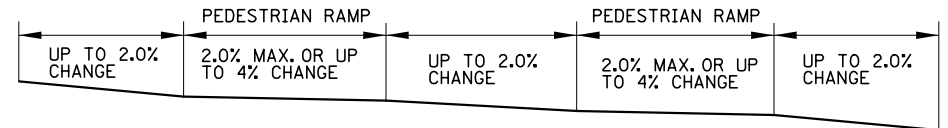
FLOW LINE PROFILE "TABLE" - TWIN PERPENDICULARS
