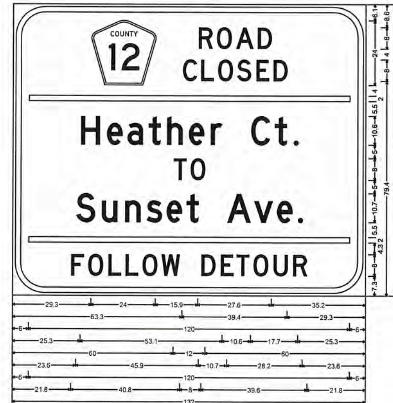
G20-X2_132x108; 12.0" Radius, 2.0" Border, 1.0" Indent, Black on Orange; [ROAD] D; [CLOSED] D; [Heather Ct.] D; [TO] D; [Sunset Ave.] D; [FOLLOW] D; [DETOUR] D;
