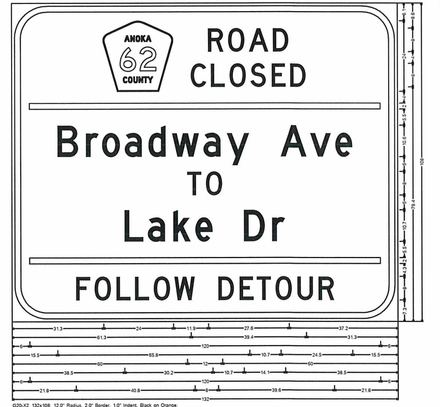
G20-X2_132x108; 12.0" Radius, 2.0" Border, 1.0" Indent, Black on Orange. [ROAD] D; [CLOSED] D; [Broadway Ave] D; [TO] D; [Lake Dr] D; [FOLLOW] D; [DETOUR] D.
