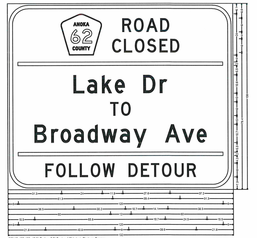
G20-X2_132x108; 12.0" Radius, 2.0" Border, 1.0" Indent, Black on Orange. [ROAD] D; [CLOSED] D; [Lake Dr] D; [TO] D; [Broadway Ave] D; [FOLLOW] D; [DETOUR] D.
