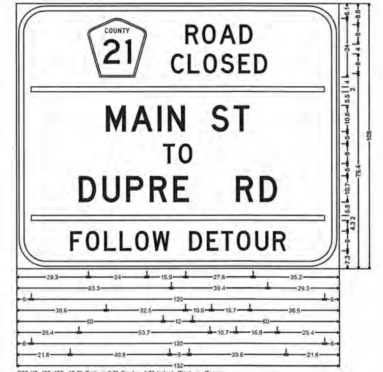
G20-X2, 132x108, 12.0" Radius, 2.0" Border, 1.0" Indent, Black on Orange; [ROAD] D; [CLOSED] D; [MAIN ST] D; [TO] D; [DUPRE RD] D; [FOLLOW] D; [DETOUR] D;
