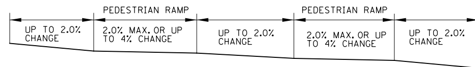
FLOW LINE PROFILE "TABLE" - TWIN PERPENDICULARS
