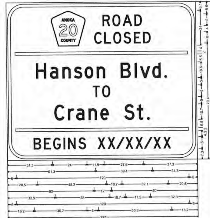
G20-X2_132x108; 12.0" Radius, 2.0" Border, 1.0" Indent, Black on Orange. [ROAD] D; [CLOSED] D; [Hanson Blvd.] D; [TO] D; [Crane St.] D; [BEGINS] D; [XX/XX/XX] D;
