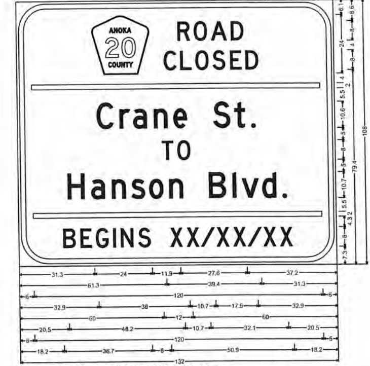
G20-X2_132x108; 12.0" Radius, 2.0" Border, 1.0" Indent, Black on Orange. [ROAD] D; [CLOSED] D; [Crane St.] D; [TO] D; [Hanson Blvd.] D; [BEGINS] D; [XX/XX/XX] D;
