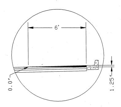
MILL 1 1/4" BELOW THE GUTTER LINE, UP TO 0" AT 6' FROM GUTTER
