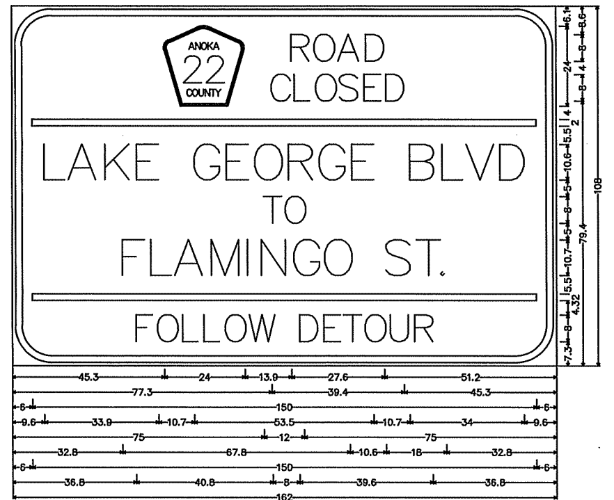
G20-X2_132x108; 12.0" Radius, 2.0" Border, 1.0" Indent, Black on Orange; [ROAD] D; [CLOSED] D; [LAKE GEORGE BLVD] D; [TO] D; [FLAMINGO ST.] D; [FOLLOW] D; [DETOUR] D;
