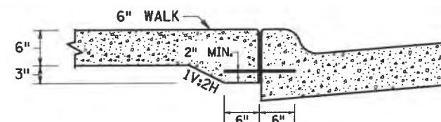
SECTION VIEW A-A THICKENED SECTION THROUGH CURB RAMP FLARES
