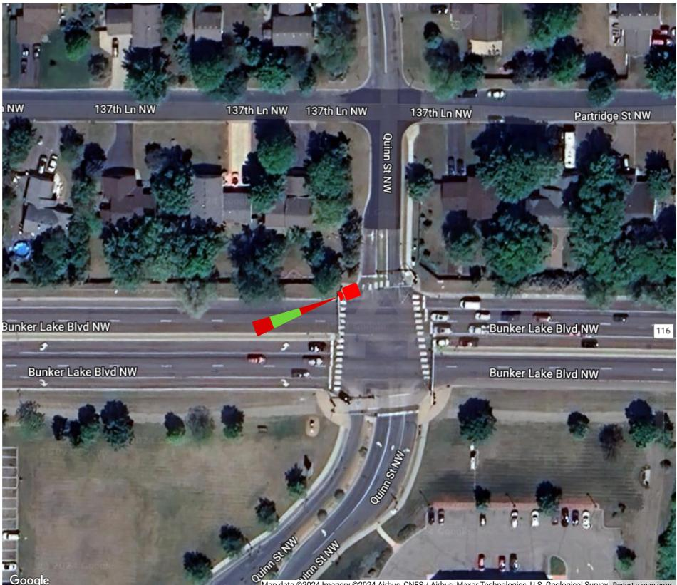
Location Notes: bucket truck traffic control horizontal extension arm mount. Traffic signals are blocking the vertical pole - horizontal installation is needed for this location.
