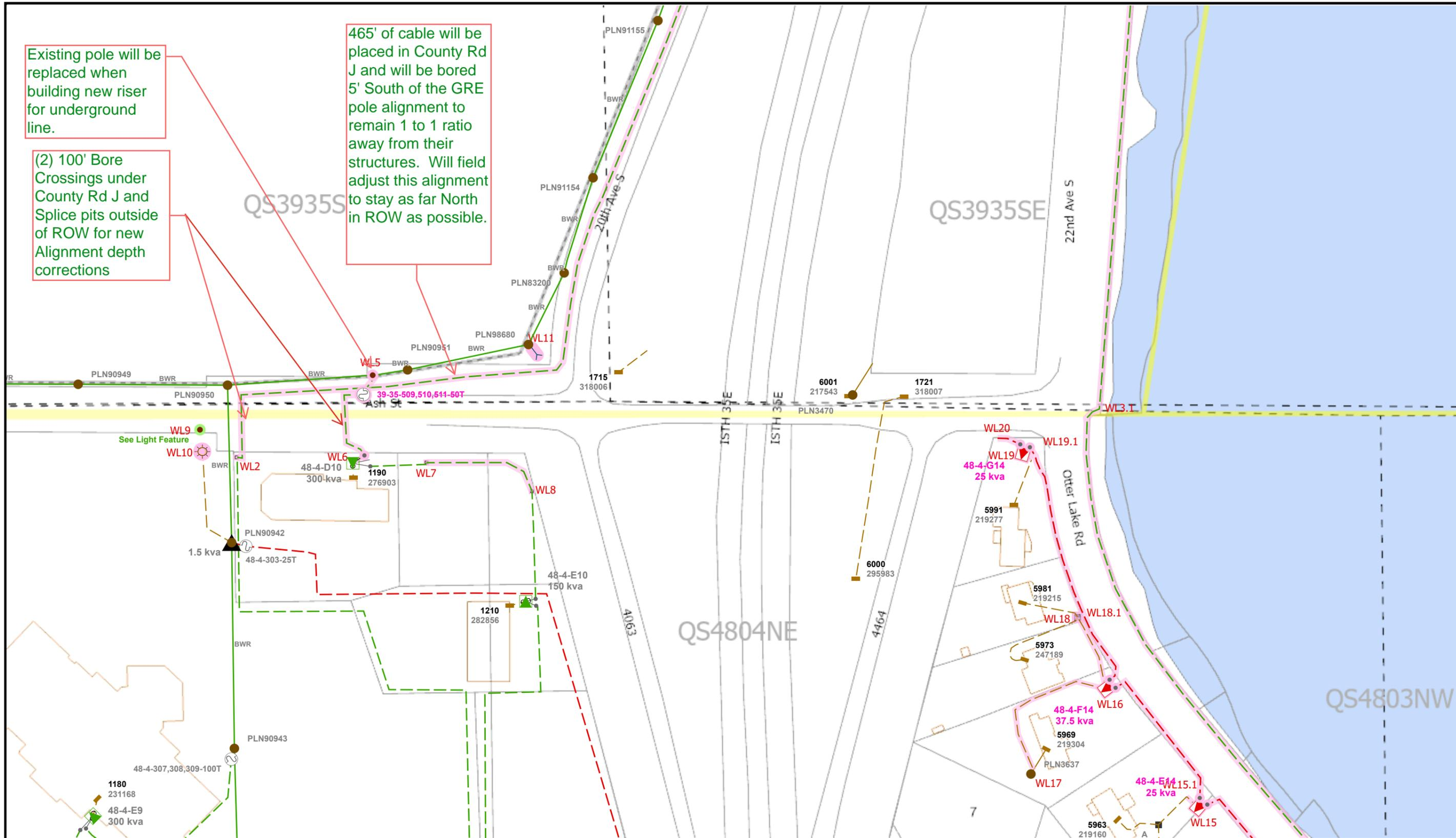
Existing pole will be replaced when building new riser for underground line.
