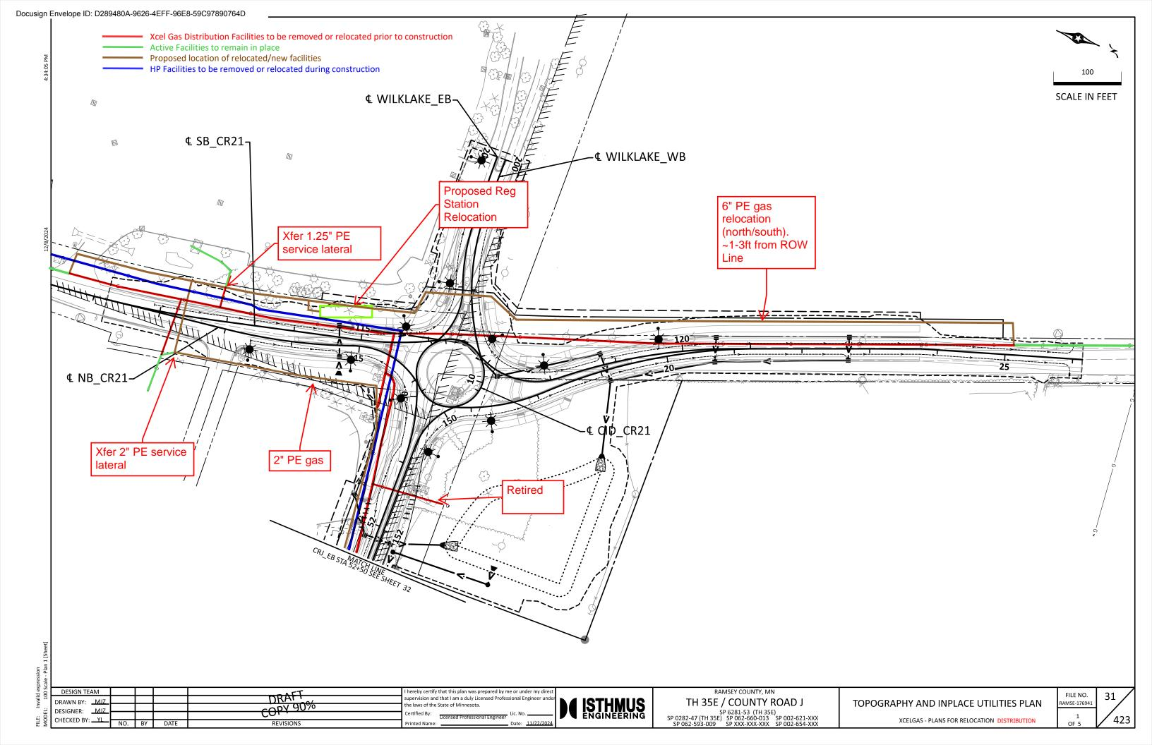
Xcel Gas Distribution Facilities to be removed or relocated prior to construction
