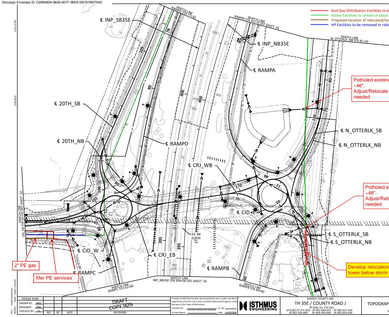
Xcel Gas Distribution Facilities to be removed or relocated prior to construction Proposed location of relocated/new facilities HP Facilities to be removed or relocated during construction
