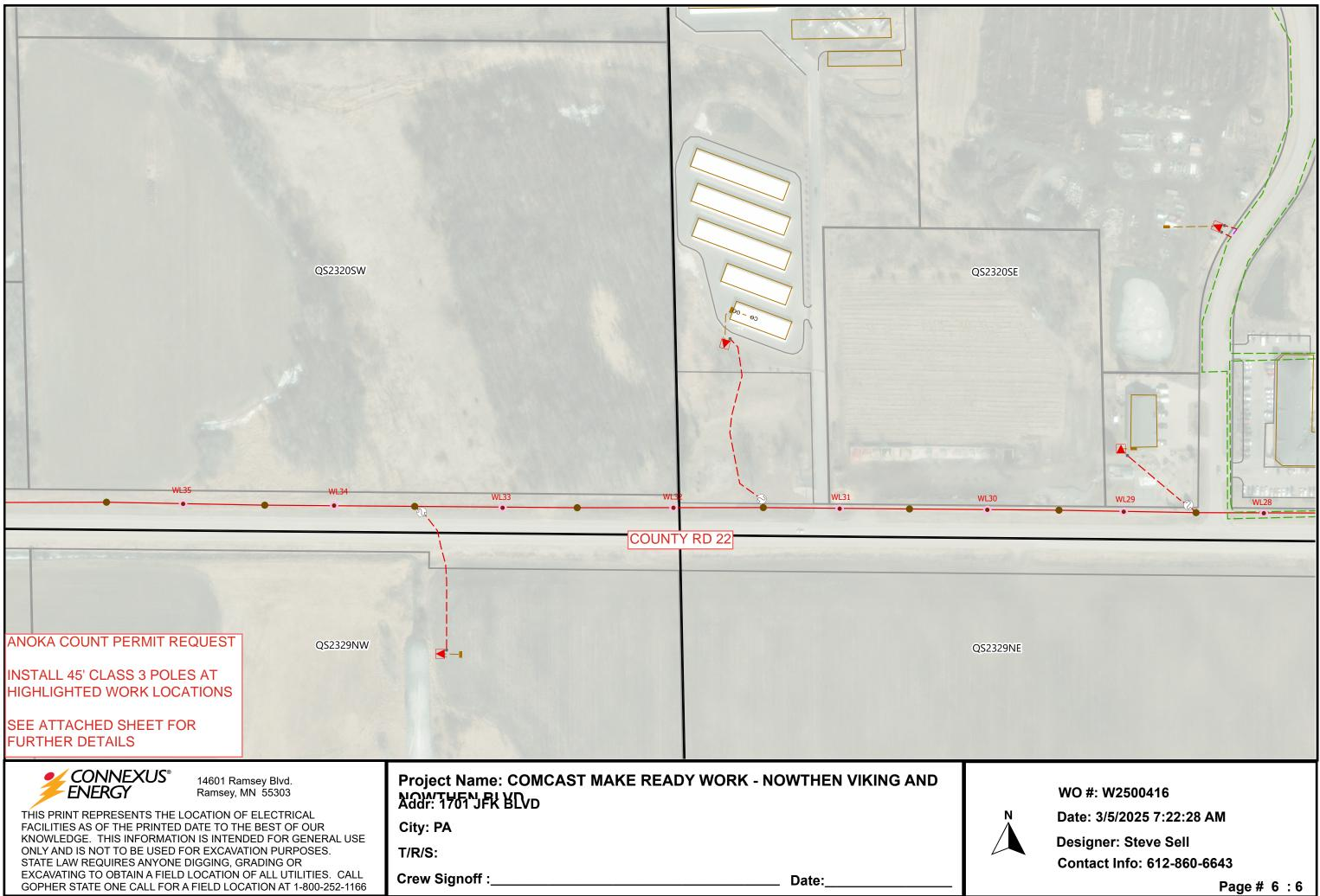
AT WL26 INSTALL 45' CLASS 3 POLE APPROXIMATELY 50' NORTH FROM CENTERLINE OF CR-22 AND 720' EAST FROM CENTERLINE OF IGUANA ST NW
