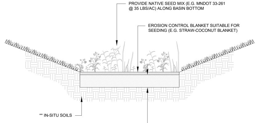
\*\* ALLEVIATE ANY COMPACTED SOILS (BY USING A PRIMARY TILLING OPERATION SUCH AS A CHISEL PLOW, RIPPER OR SUBSOILER) TO A DEPTH NECESSARY TO ALLEVIATE COMPACTION
