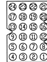
FRONT VIEW OF J1 HARNESS (SWITCH PANEL)
