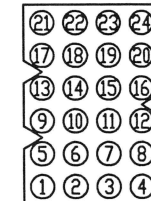
FRONT VIEW OF J1 JACK (SWITCH PANEL)
