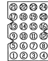
FRONT VIEW OF J1 JACK (SWITCH PANEL)
