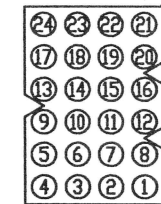
FRONT VIEW OF J1 HARNESS (SWITCH PANEL)
