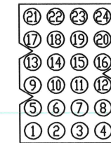
FRONT VIEW OF J1-J6 HARNESSES (POWER BUS PANEL)
