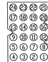
FRONT VIEW OF J1 JACK (SWITCH PANEL)
