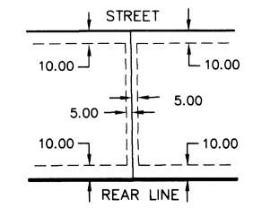
BEING 5 FEET IN WIDTH AND ADJOINING SIDE LOT LINES, AND 10 FEET IN WIDTH AND ADJOINING STREET LINES AND REAR LOT LINES, UNLESS OTHERWISE SHOWN ON THE PLAT
