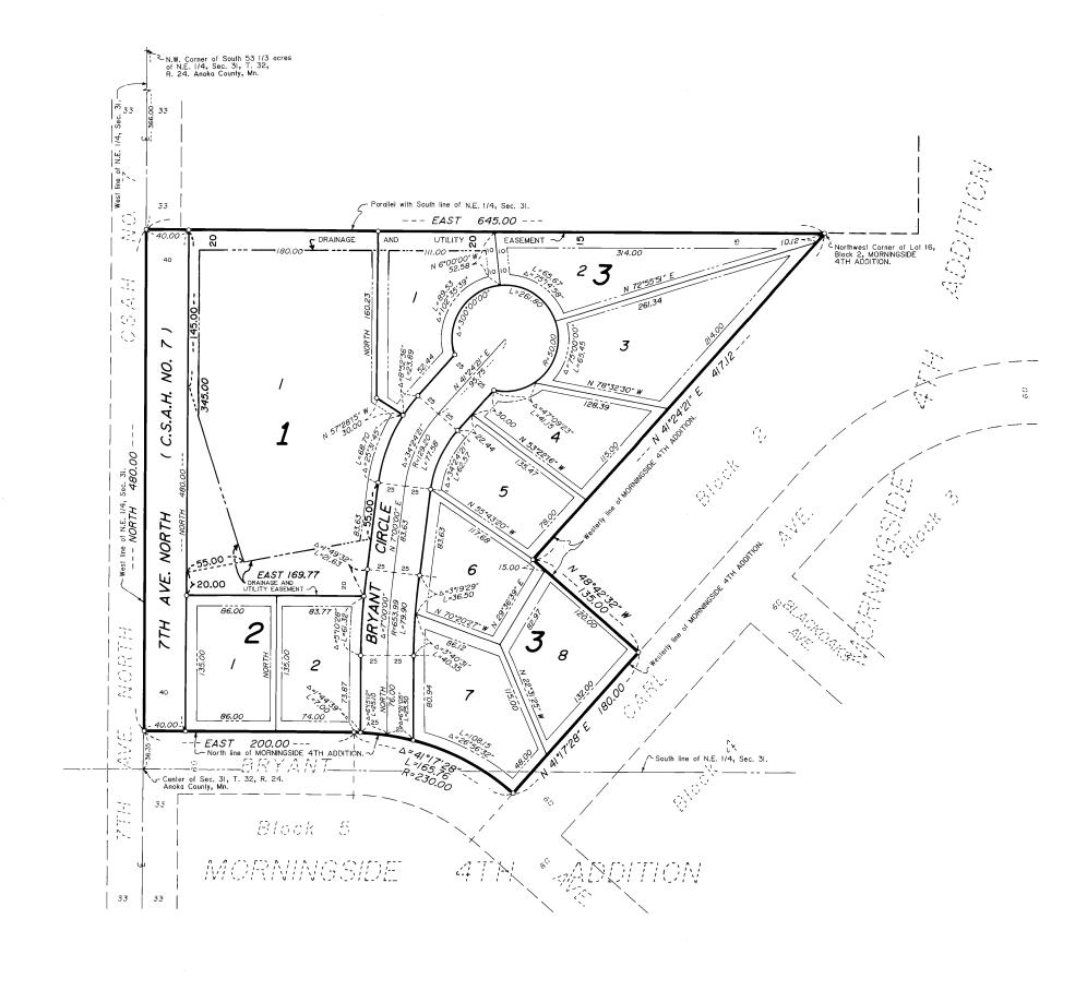
Scale : I inch = 100 feet. For the purposes of this plat, the West line of the N.E. 1/4 of Sec. 31 is assumed to bear NORTH. O Denotes iron pipe set with a plastic plug stamped RLS 13057. Drainage and Utility Easements are shown thus : Based upon State Plane Coordinates by Anoka County Surveyor.
