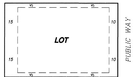
BEING 5 FEET IN WIDTH AND ADJOINING SIDE LOT LINES, BEING 10 FEET IN WIDTH AND ADJOINING PUBLIC WAYS AND BEING 15 FEET IN WIDTH AND ADJOINING REAR LOT LINES, UNLESS OTHERWISE SHOWN ON THIS PLAT.
