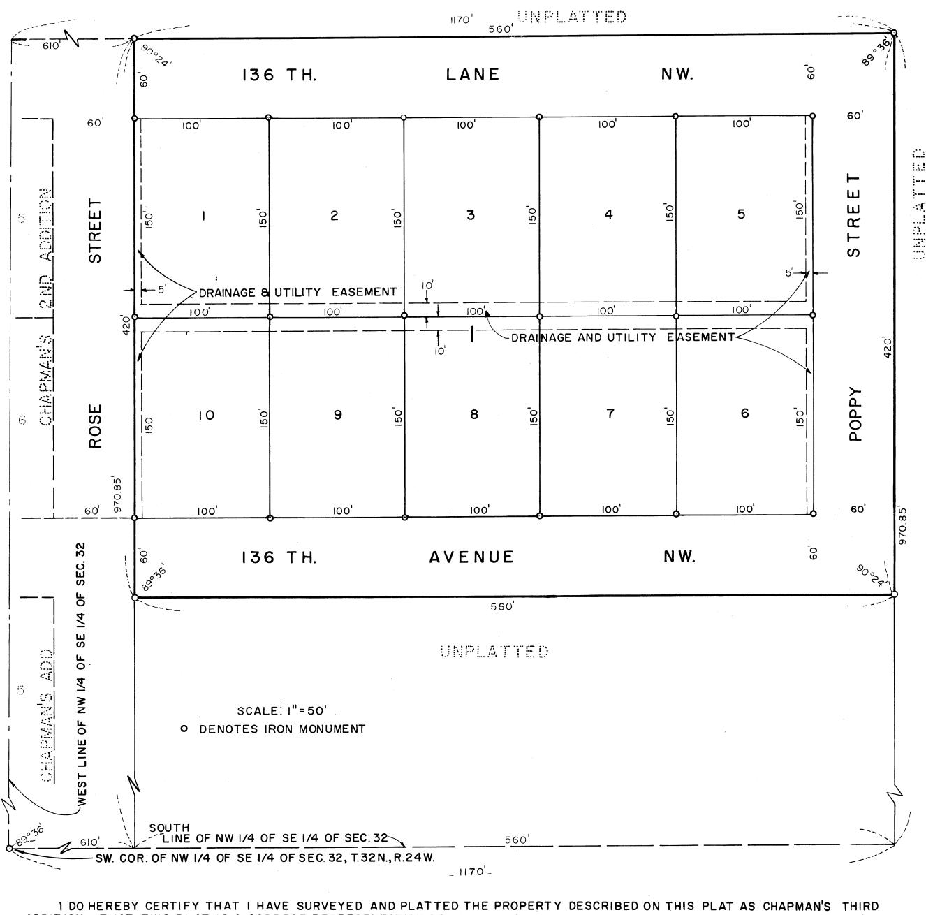
ADDITION; THAT THIS PLAT IS A CORRECT REPRESENTATION OF SAID SURVEY; THAT ALL DISTANCES ARE CORRECTLY SHOWN ON SAID PLAT IN FEET AND DECIMALS OF A FOOT; THAT THE MONUMENTS FOR THE GUIDANCE OF FUTURE SURVEYS HAVE BEEN CORRECTLY PLACED IN THE GROUND AS SHOWN ON THE PLAT; THAT THE OUTSIDE BOUNDARY LINES ARE CORRECTLY DESIGNATED ON THE PLAT; AND
