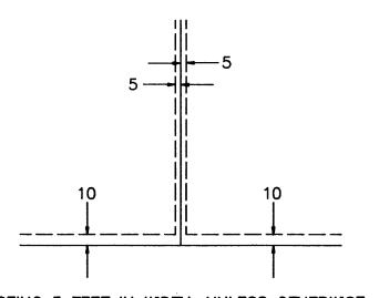
BEING 5 FEET IN WIDTH, UNLESS OTHERWISE INDICATED, AND AJOINING LOT LINES, AND 10 FEET IN WIDTH AND ADJOINING STREET LINES, AS SHOWN ON PLAT.
