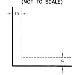
Being 10 feet in width and adjoining right—of—way lines unless otherwise shown.
