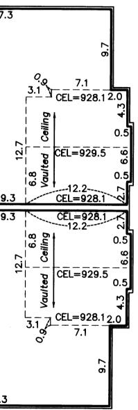
All Sidewalks, and Patios are LIMITED COMMON ELEMENTS assigned to the UNIT adjoining thereto. L.C.E. – Denotes Limited Common Element Elevations shown are referenced to a bench mark as denoted on Sheet 1 of 2 Sheets. All inside finished surface to inside finished surface dimensions and elevations are shown in feet and tenths of a foot. SW — Denotes Sidewalk CEL - Denotes Ceiling Elevation
