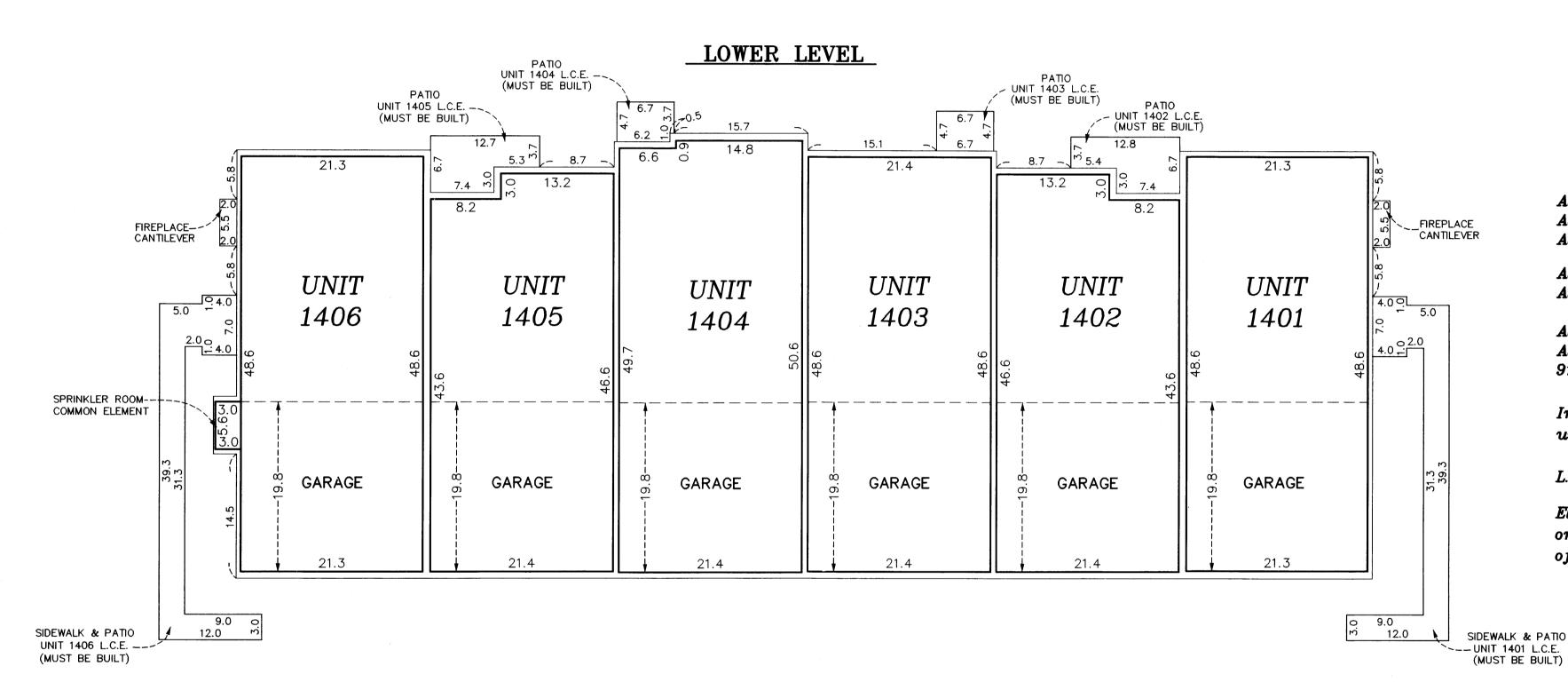
All units garage floor elevation at the garage door = 899.9 feet All units garage floor elevation at back of garage= 900.2 feet All units garage ceiling elevations = 909.5 feet
