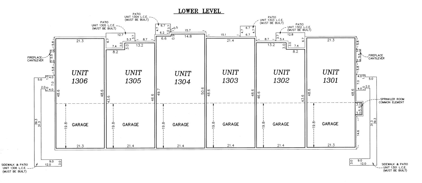
All units garage floor elevation at the garage door = 899.7 feet All units garage floor elevation at back of garage= 900.0 feet All units garage ceiling elevations = 909.3 feet
