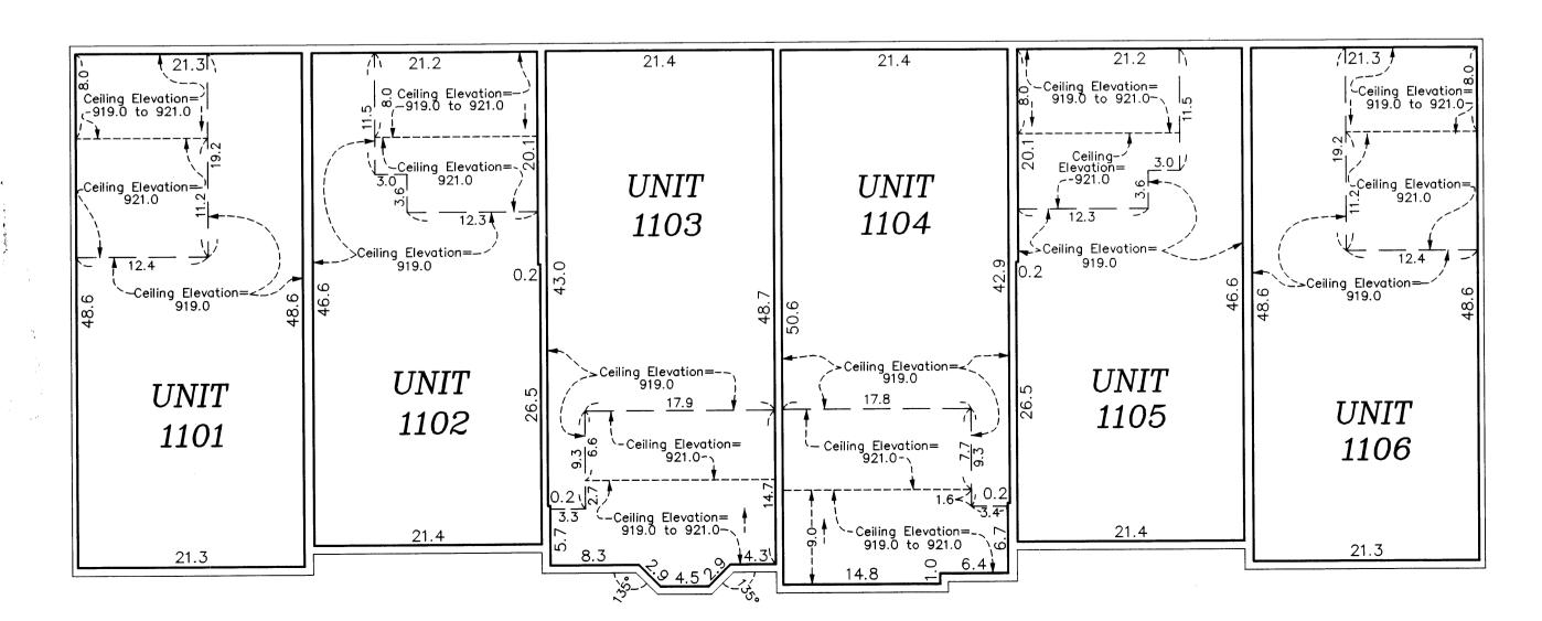
All units garage floor elevation at the garage door = 899.7 feet All units garage floor elevation at back of garage= 900.0 feet All units garage ceiling elevations = 909.3 feet
