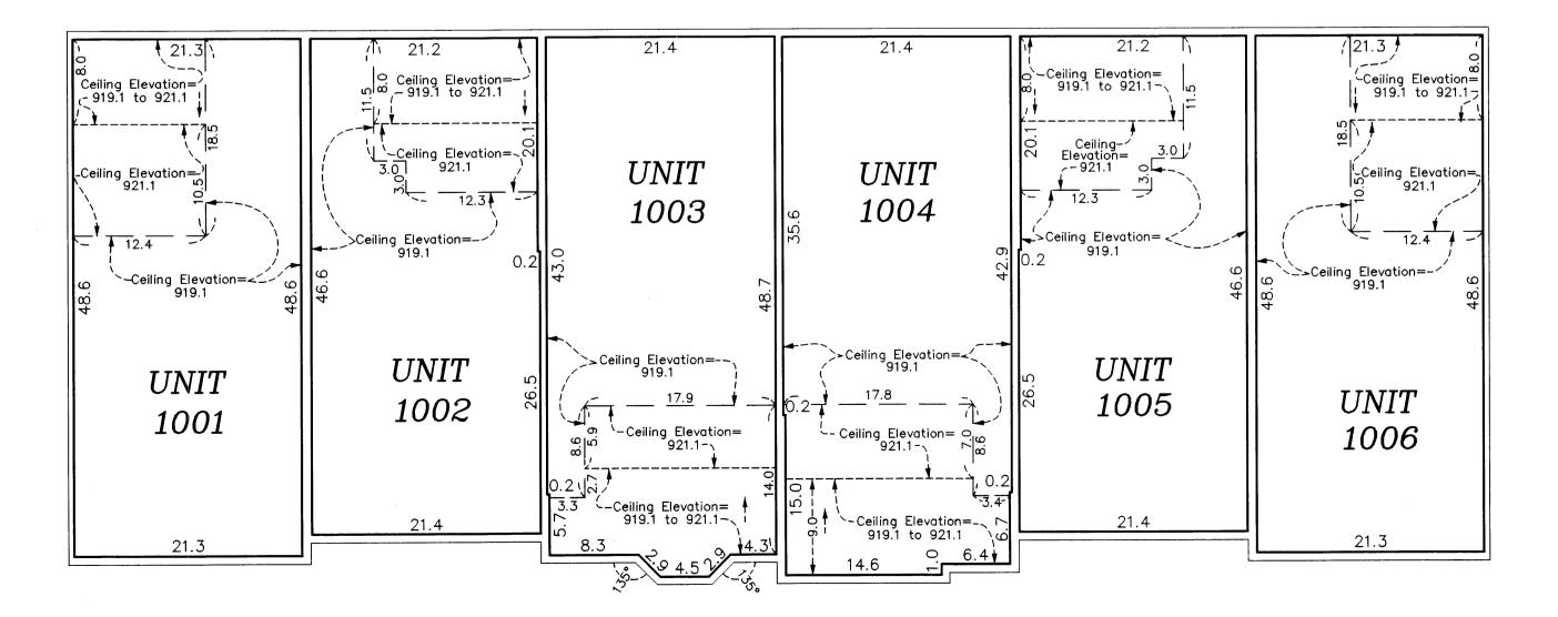
All units garage floor elevation at the garage door = 899.8 feet All units garage floor elevation at back of garage= 900.1 feet All units garage ceiling elevations = 909.4 feet
