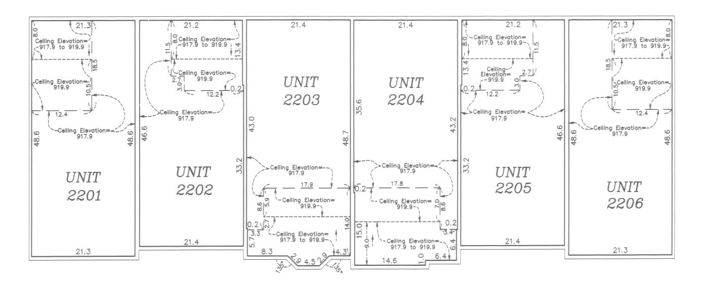
All units garage floor elevation at the garage door = 898.6 feet
