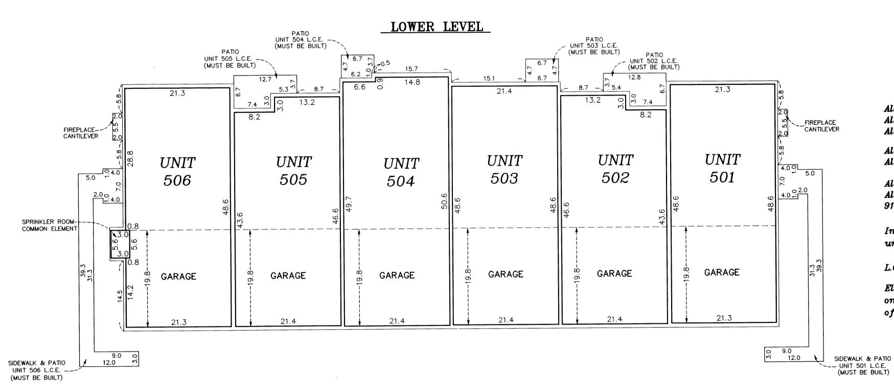
All units garage floor elevation at the garage door = 898.5 feet All units garage floor elevation at back of garage= 898.8 feet All units garage ceiling elevations = 908.1 feet
