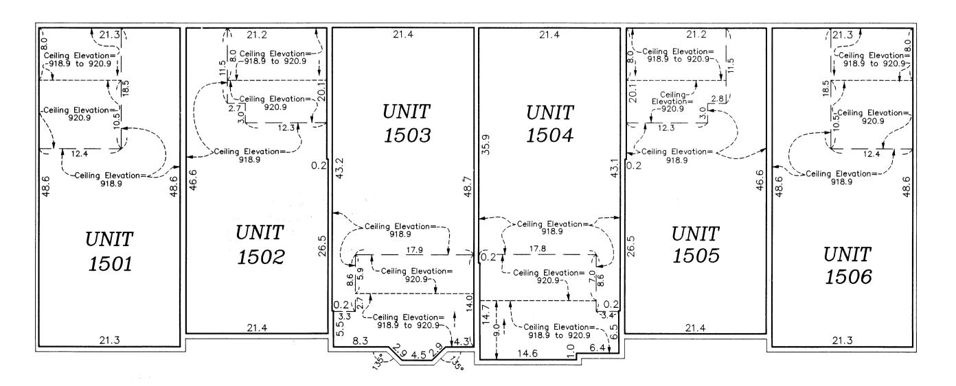
All units garage floor elevation at the garage door = 899.6 feet All units garage floor elevation at back of garage= 899.9 feet All units garage ceiling elevations = 909.2 feet
