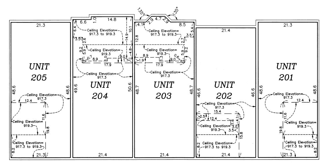
All units garage floor elevation at the garage door = 898.0 feet
