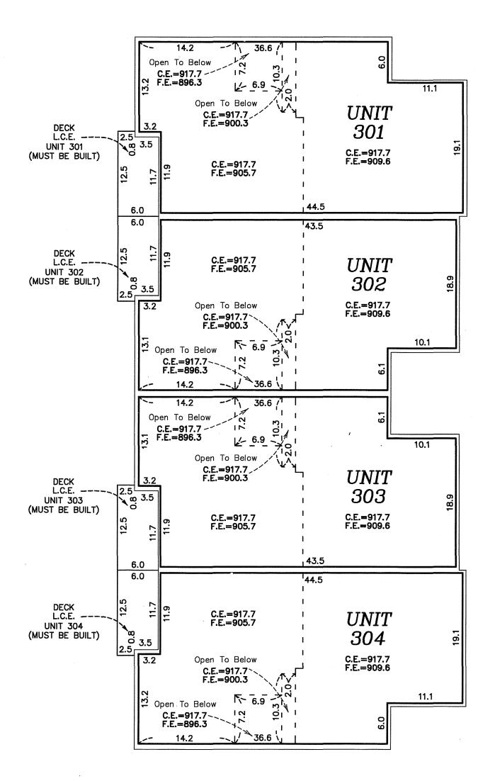
Elevations are referenced to a benchmark as noted on the site plan on Sheet 1 of 3 Sheets and are shown in feet and tenths of a foot.
