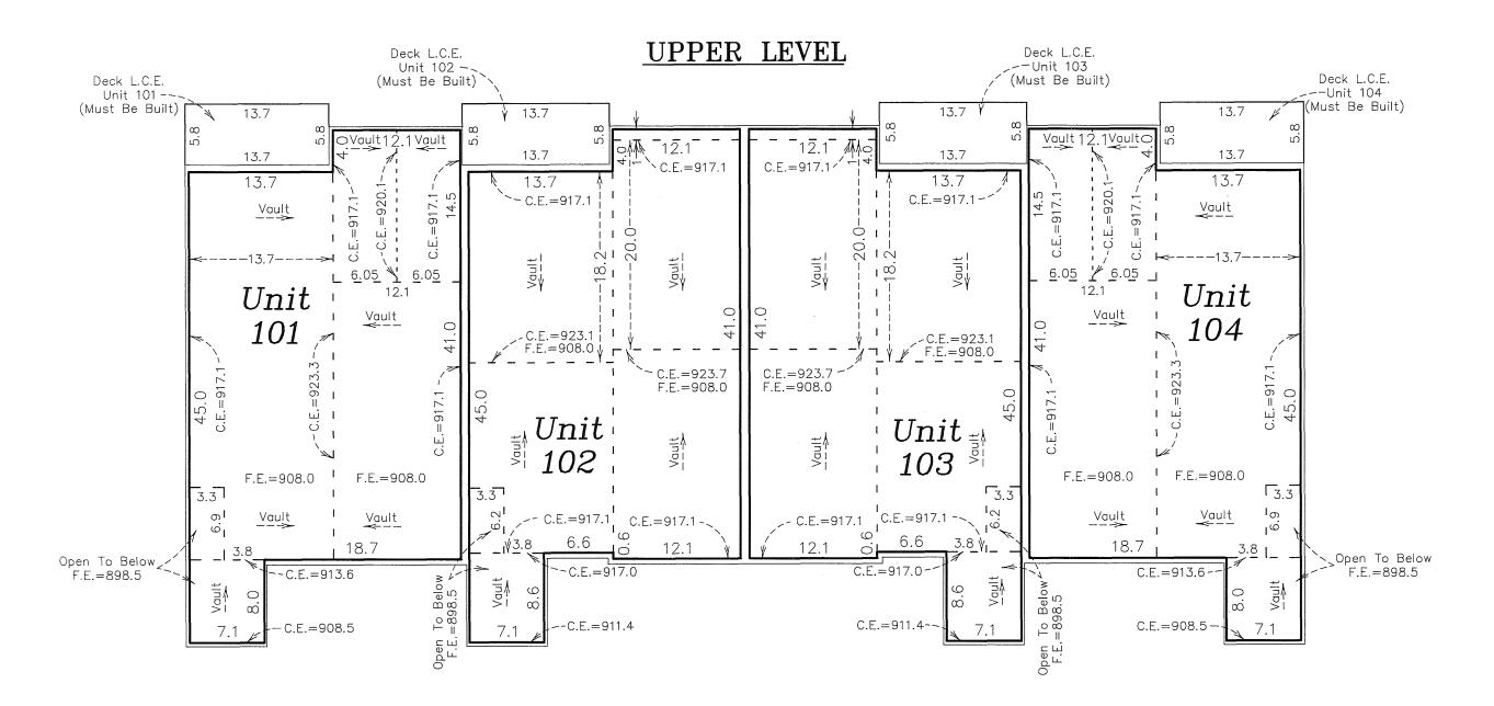
Elevations are referenced to a benchmark as noted on the site plan on Sheet 1 of 3 Sheets and are shown in feet and tenths of a foot.
