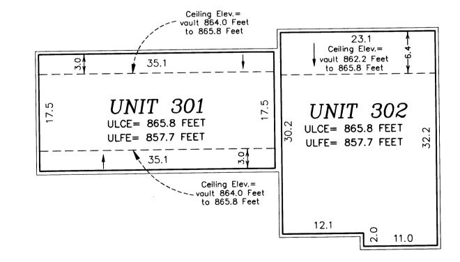
Garage Floor Elevation = GFE Garage Ceiling Elevation = GCE Lower Level Floor Elevation = LLFE Lower Level Ceiling Elevation = LLCE Upper Level Floor Elevation = ULFE Upper Level Ceiling Elevation = ULCE
