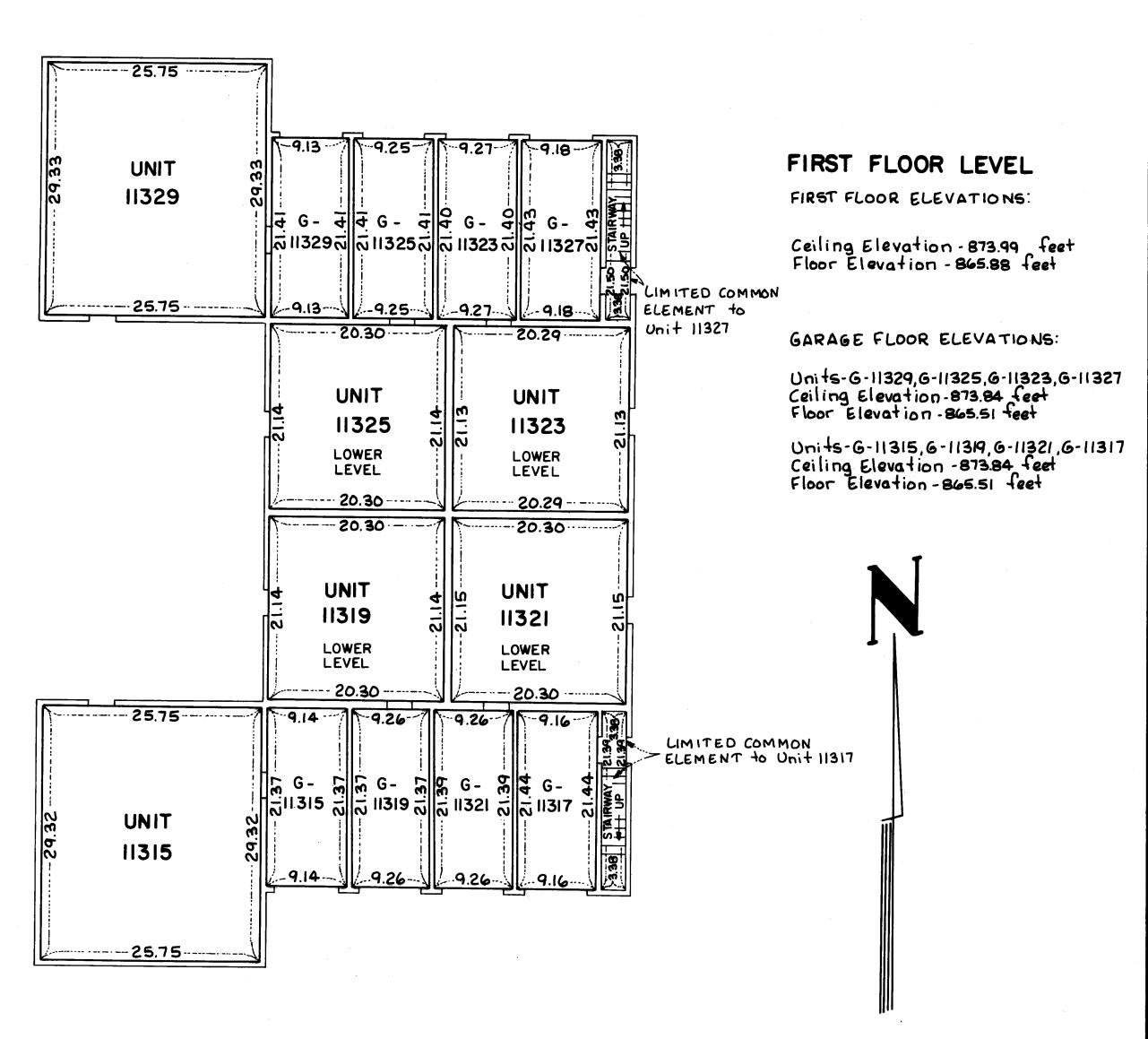
Elevations shown are referenced to a Benchmark shown on the Site Plan.
