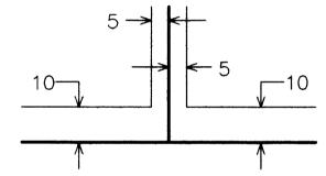
BEING 10 FEET IN WIDTH AND ADJOINING RIGHT-OF-WAY LINES, AND BEING 5 FEET IN WIDTH AND ADJOINING LOT LINES, UNLES OTHERWISE SHOWN ON THE PLAT.
