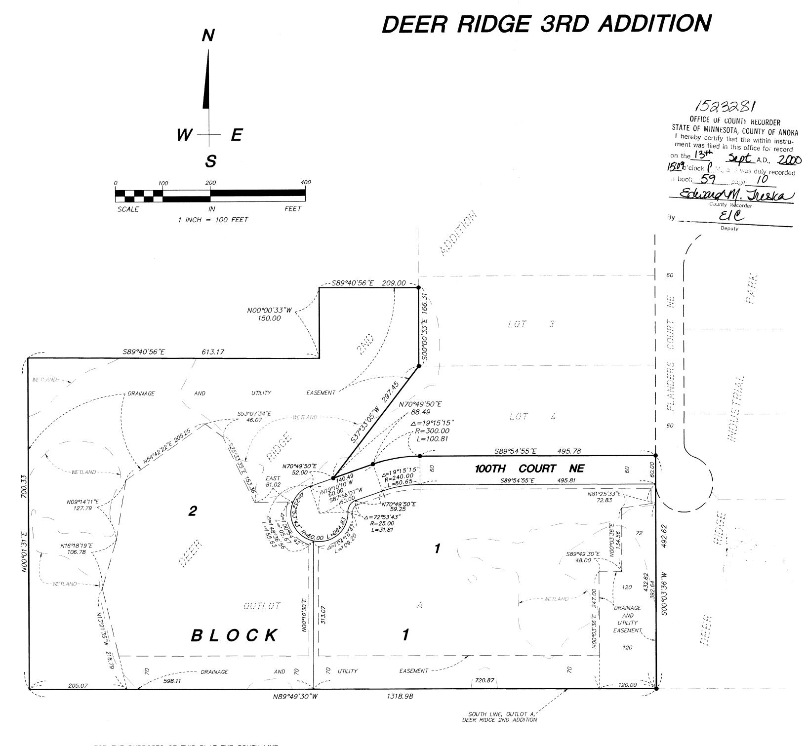
FOR THE PURPOSES OF THIS PLAT THE SOUTH LINE OF OUTLOT A, DEER RIDGE 2ND ADDITION IS ASSUMED TO HAVE A BEARING OF SOUTH 89 DEGREES 49 MINUTES 30 SECONDS EAST.
