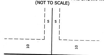
BEING 10 FEET IN WIDTH TO RIGHT OF WAY LINES, AND 5 FEET IN WIDTH TO ADJOINING LOT LINES UNLESS OTHERWISE SHOWN ON THIS PLAT.
