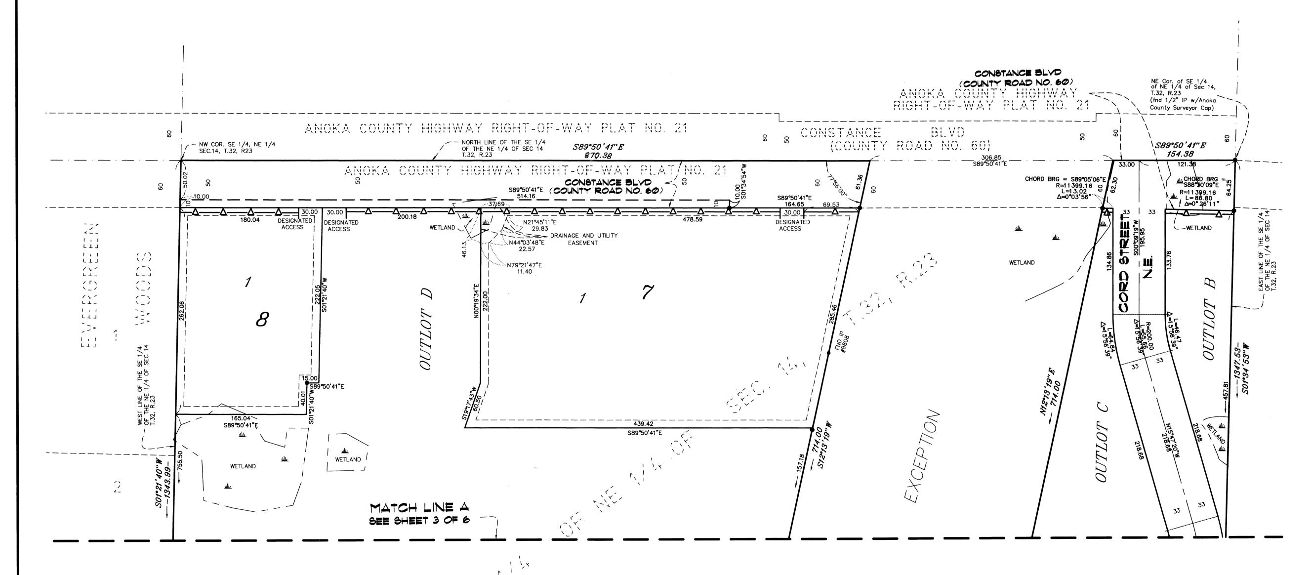
All monuments required by Minnesota Statute, and not shown on this plat, will be set within one year of the recording date of this plat, and shall be evidenced by a 1/2 inch by 18 inch iron pipe marked by RLS 41578.
