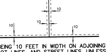
BEING 10 FEET IN WIDTH ON ADJOINING LOT LINES, AND STREET LINES, UNLESS OTHERWISE SHOWN ON THE PLAT.
