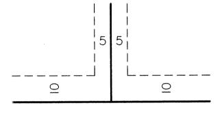
BEING 5 FEET IN WIDTH, AND ADJOINING LOT LINES, AND IO FEET IN WIDTH AND ADJOINING RIGHT OF WAY AND REAR LOT LINES UNLESS OTHERWISE SHOWN ON THE PLATE
