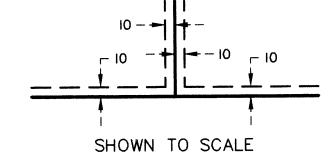
BEING IO FEET IN WIDTH AND ADJOINING LOT LINES, AND RIGHT OF WAY LINES, UNLESS OTHERWISE INDICATED ON THIS PLAT.
