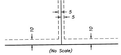
Being 5 feet in width, and adjoining lot lines, and 10 feet in width and adjoining street right—of—way lines unless otherwise shown on the plat.
