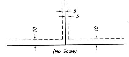
Being 5 feet in width, and adjoining lot lines, and 10 feet in width and adjoining street right—of—way lines unless otherwise shown on the plat.
