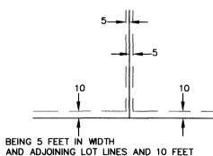
AND ADJOINING LOT LINES AND 10 FEET IN WIDTH AND ADJOINING RIGHT OF WAY LINES UNLESS OTHERWISE SHOWN ON THE PLAT.
